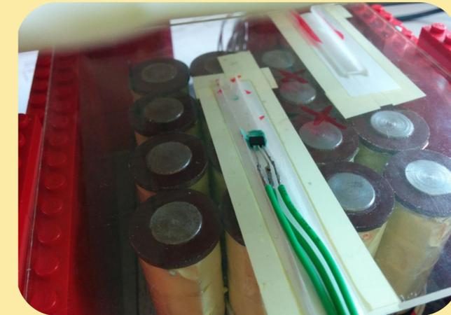
A groove was cut into the Perspex buffer and the hall effect sensor was fitted, flush with the buffer
