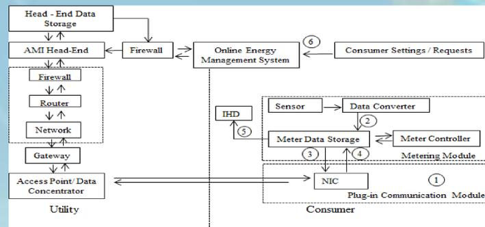
Figure 1: Consumer Oriented Smart Metering System Architecture
