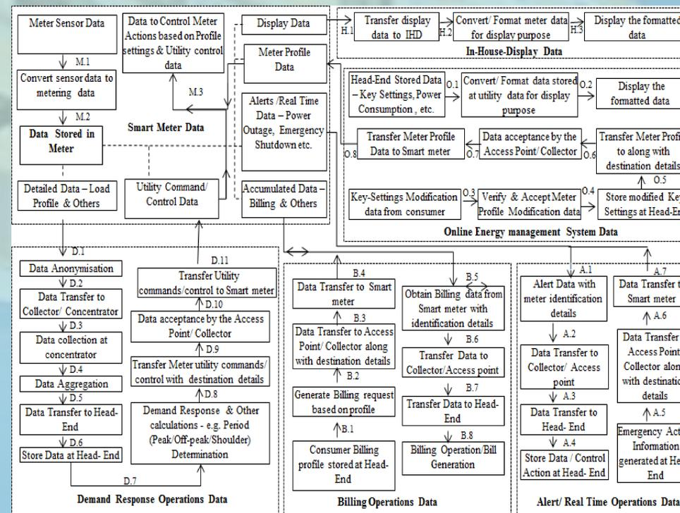
Figure 2: Abstract Data Flow Model for Smart Metering System
